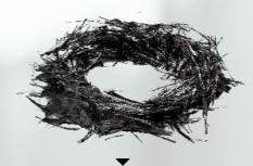
Recycled Carbon Fiber Paper produced by Thermolysis, using recycled carbon fiber
